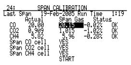
Verify span gas values to Cal Cylinder.
