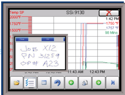
Built in Chart Recorder with Notes
