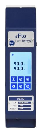
eFlo 2.0 can operate in Flow mode or Valve mode (options not available with Manual meters).
