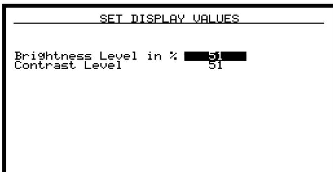
This page is used to adjust the display backlight brightness and the contrast. The values entered range from 0 to 100.
