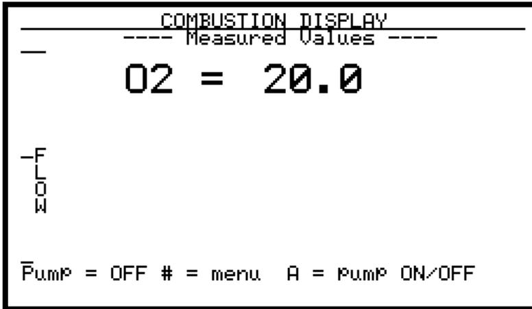
The combustion display shows the current reading in % excess oxygen. Also shown is the relative flow rate of the sample by a fuel gauge on the left-hand side of the screen. The sample pump may be turned on or off by pressing the **A** key.
