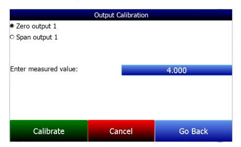
The user will then measure the current at the appropriate output terminals and enter that value into the blue box by tapping on it once to bring up a number pad. Save this value by pressing **OK**.
