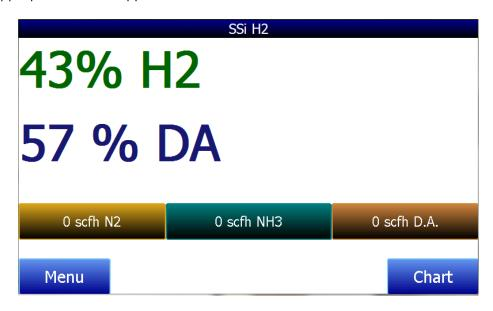
The home screen also displays the flow of  $N_2$ ,  $NH_3$ , and D.A. These values can be entered by the operator when the instrument is in the mode to evaluate Kn or %DA. This is discussed further under the Instrument Configuration section. The **Menu** button in the bottom left-hand corner will take the operator to the configurable options within the controller. The **Chart** button in the bottom right-hand corner of the screen will display the data trend chart.
