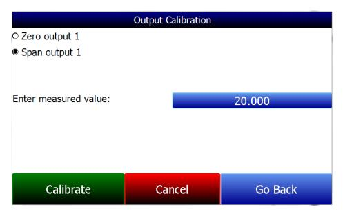
The user will then measure the current at the appropriate output terminals and enter that value into the blue box by tapping on it once to bring up a number pad. Save this value by pressing **OK**.
