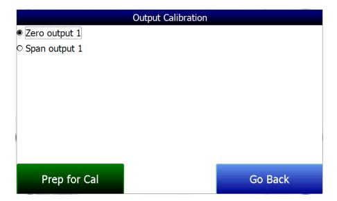
The Portable  $H_2$  has one 4-20 mA output. For optimal accuracy the output can be verified and if necessary calibrated.
