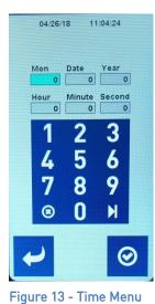
Use the numeric keypad to set the date and time of the device.
