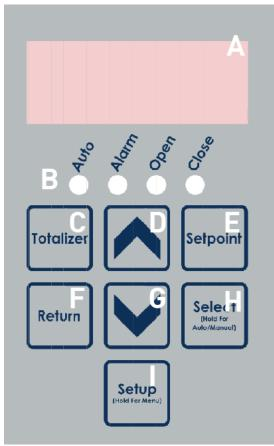
Figure 4 - eFlo 2.0 LED Flow Control Panel Layout
