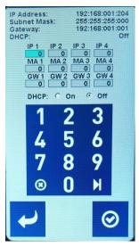
Values are modifiable and are used to set the Ethernet Settings.
