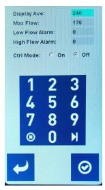
**Display Average** – Increasing this value will increase the average of the flow rate being displayed on the main screen (range for this value is 1 to 255)
